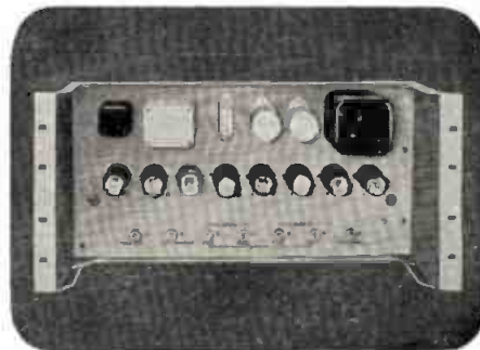
RCA GENLOCK, Type TG-45. This is the simple, automatic system that electrically locks two separate television pick-up systems together.
